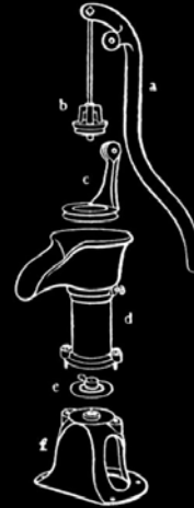
Cast-iron House- pump. — a , lever; b , plunger or piston; c , fulcrum; d , cylinder or barrel; e , lower valve, or foot-valve; f , base, supporting all other parts.
